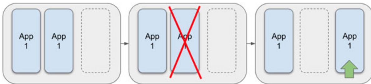
Figure 9.11: When a container in the cluster crashes, Kubernetes can create a new instance to replace it.
